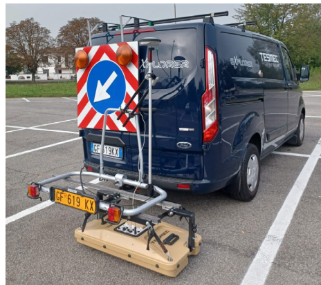
Explorer 3.0 – vehicle pulled in "mobile" configuration
