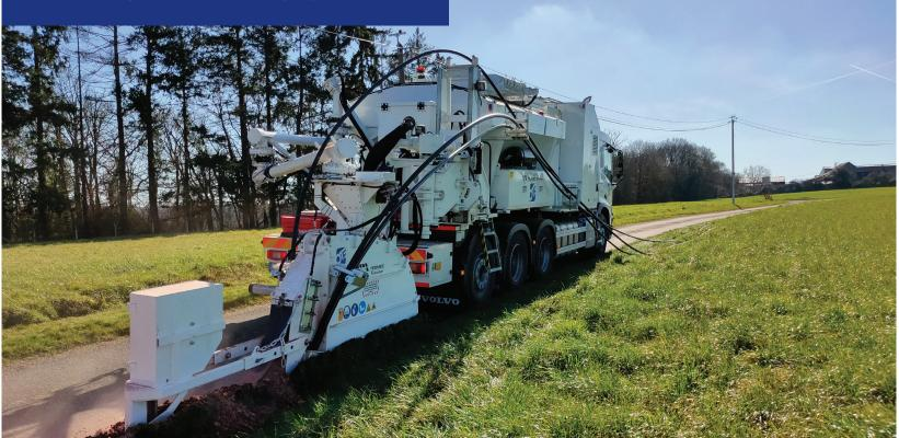
Greenpose is the innovative solution for fiber optic deployment in extra-urban areas, including trenching, cleaning of the ditch, treatment of excavated material and reutilization of the excavated materials as backfill
