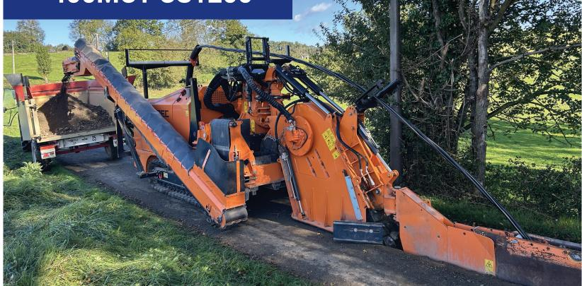
Tesmec 400MCT with CS1200 is a 15 metric ton-class trencher featuring a 238 Hp (175 kW) tier 4 engine/ Stage V, or a 218 Hp (160 kW) tier 3 engine, designed for telecom and energy cables projects in urban and extra-urban areas
