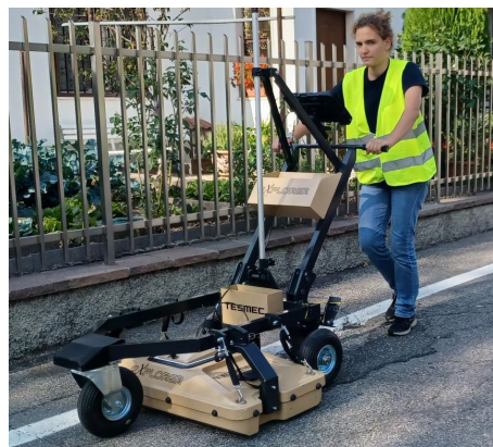
Explorer 3.0 – vehicle pulled in “trolley” configuration
