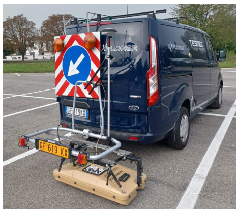
Explorer 3.0 – vehicle pulled in “mobile” configuration
