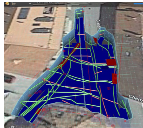
The image shows the reconstruction of a detected underground network
